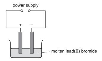
An element is produced at the negative electrode.
