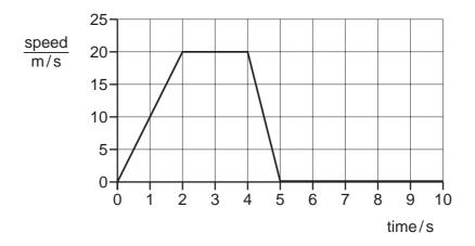
Between which times does the car have the most kinetic energy?
